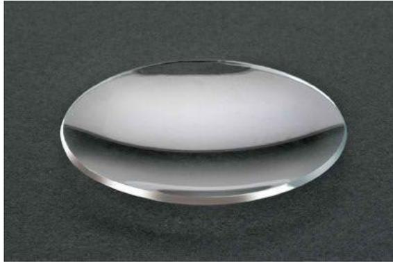
*Gambar 9. Kaca arloji ( Sumber : [www.abprospecting.com](http://www.abprospecting.com) )*
